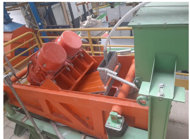
Fig. 2. Laboratory screen installation with slurry feeder and vibrating mechanism.
